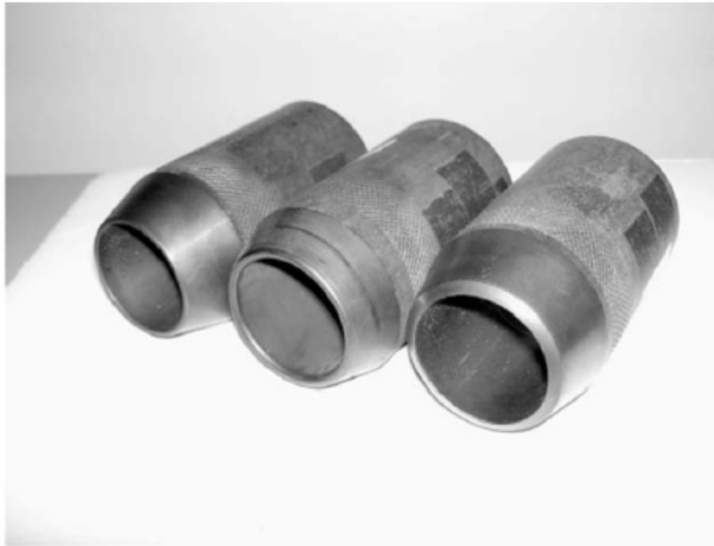
Drive samplers usually employ three types of cutting heads, or shoes, shown here. The sharp tapered heads are intended for soil sampling, while the more blunt tips are designed for greater longevity when sampling granular soils.
